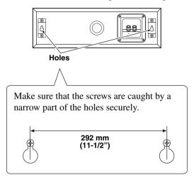
Fasten screws into a firm wall or wall support as shown in the figure below, and hang the holes on the protruding screws.
