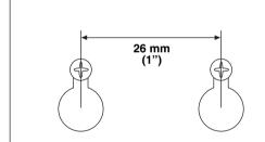
Fasten screws into a firm wall or wall support as shown in the figure below, and hang the holes on the protruding screws.
